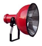
**2.GLASS** reflector: High intensity long range weather proof (IP65), symmetrical beam flood light, the front housing should have made of low carbon aluminum alloy with cast alu. back housing, the main reflector is in glass with SS side reflector for maximum output of lux, 5 mm thick toughened front glass with endless neoprene rubber gasket, E-40 lamp holder, body would be painted by powder coating epoxy, separate control gear for suitable for HPSV or MH lamp of 150/250/400/1000 watt.
