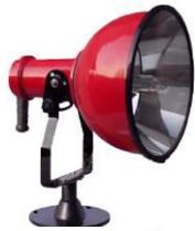
**1. LRF model with Alu. body & GLASS reflector:** High intensity search cum flood light, the front housing should have made of thick Aluminum alloy with cast back housing, the main reflector is in glass with SS side reflector, 5 mm thick toughened front glass with endless neoprene rubber gasket, E-40 lamp holder, painted by powder coating epoxy, separate control gear for HPSV or MH lamp of 250/400/1000 watt (lamp life is appx 30,000 burning hrs).
